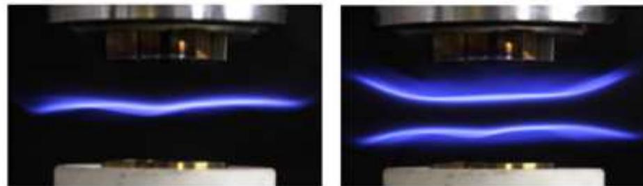
Images of a single (left) and twin (right) counterflow burner flames
