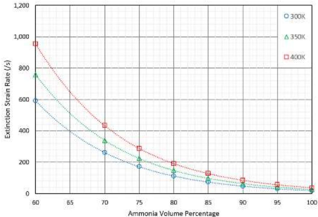
Calculated Extinction Strain Rate – Ammonia/Hydrogen blend with Air vs Nitrogen, 25mm BSD, 300K Preheat, Nakamura kinetic mechanism
