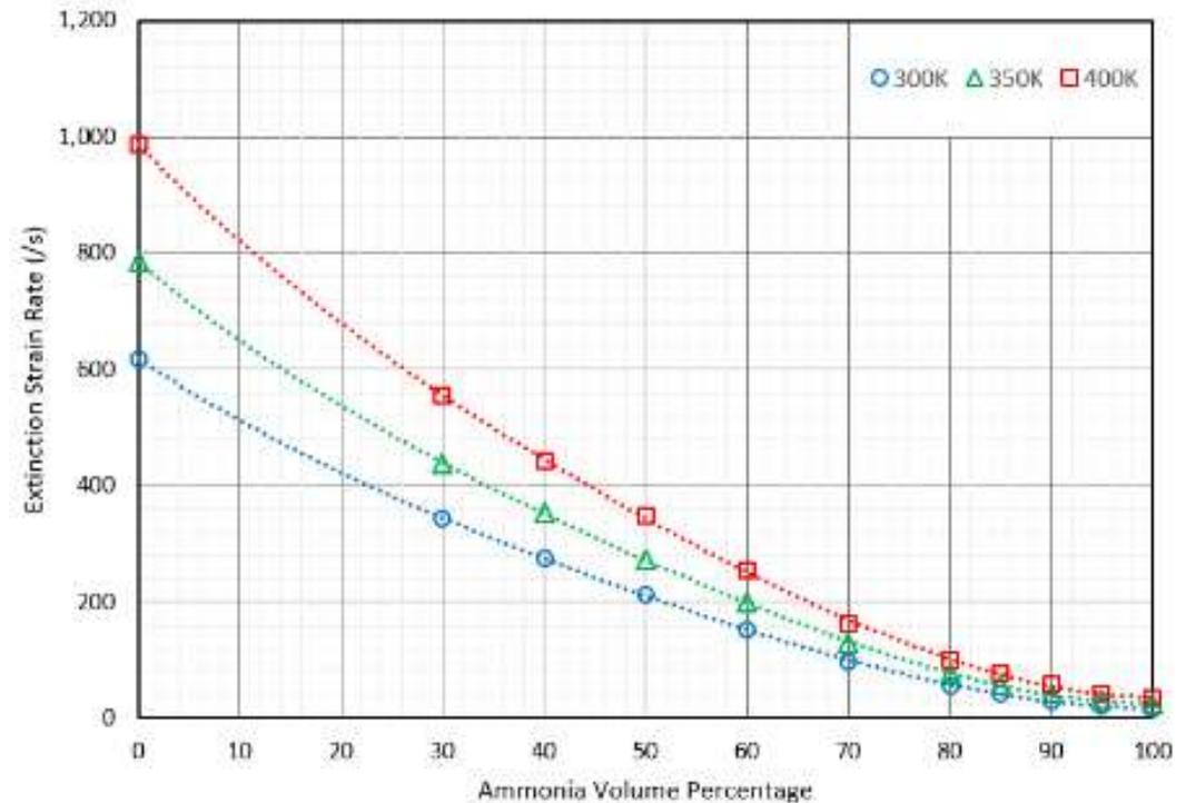
Calculated Extinction Strain Rate – Ammonia/Methane blend with Air vs Nitrogen, 25mm BSD, 300K Preheat, Arunthanayothin kinetic mechanism
