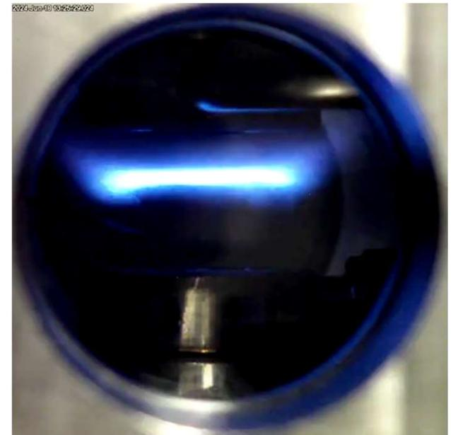
Example of counterflow flame extinction - Premix methane/air vs nitrogen, ER 1.05, 350K
