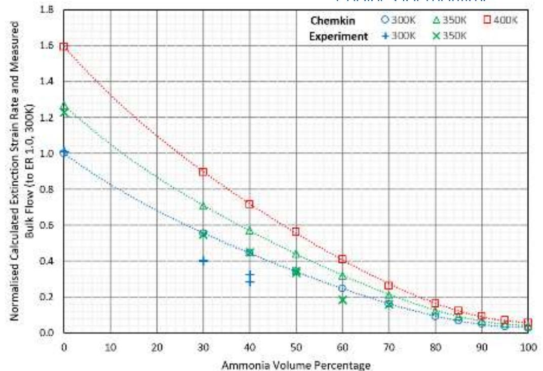
Calculated and Experimental Extinction Values Premix Ammonia/Methane and Air vs Nitrogen.
