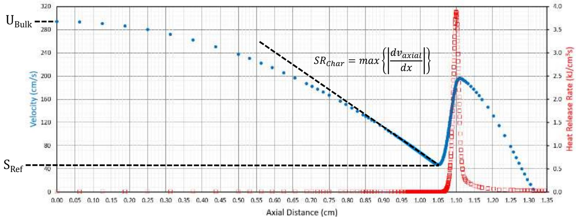
Determination of Characteristic Strain and Reference Flame Speed from counterflow burner velocity profile
