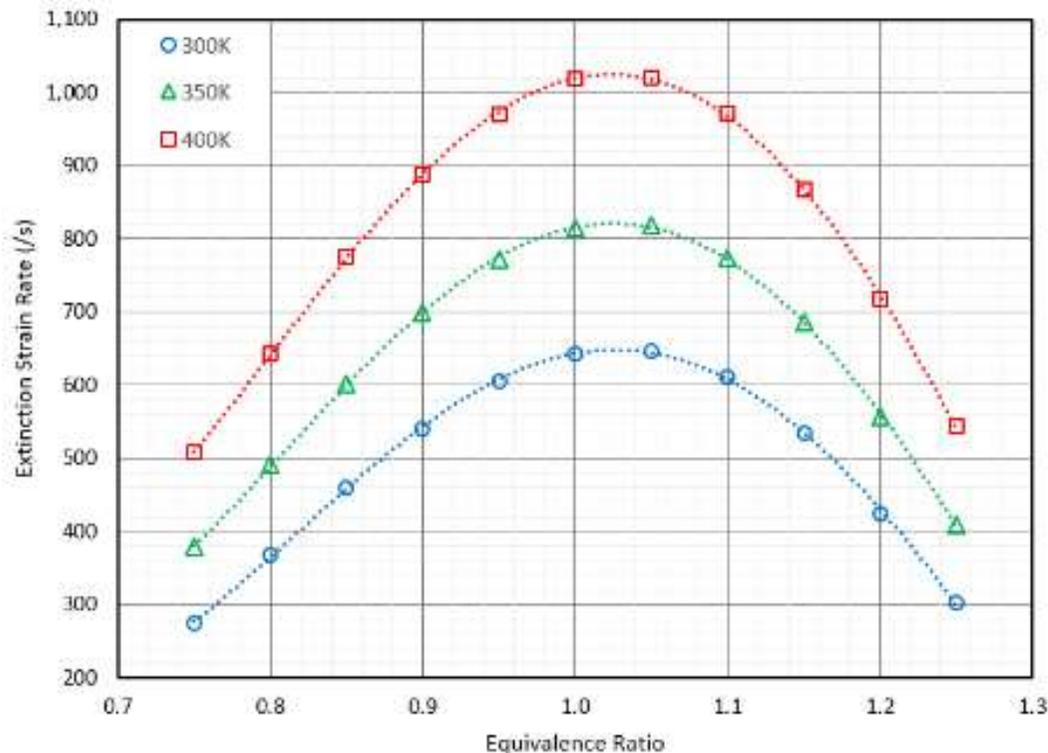
Calculated Extinction Strain Rate – Premix Methane and Air vs Nitrogen, 25mm BSD, 300K Preheat, Gri-Mech 3.0 kinetic mechanism
