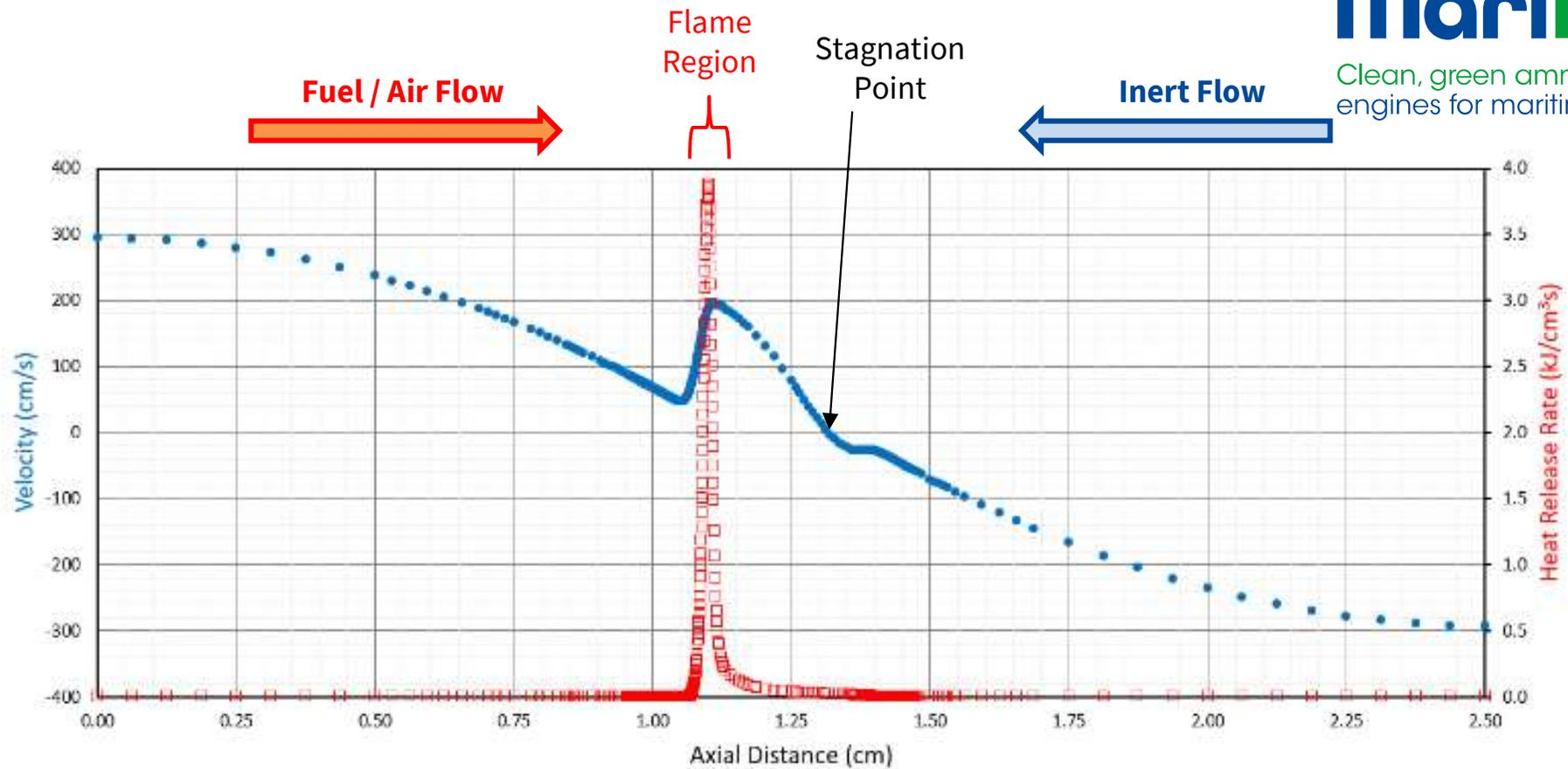
Chemkin simulation of a stable, stoichiometric premixed (single) methane flame – 25mm BSD, 300K Preheat, Gri-Mech 3.0 kinetic mechanism
